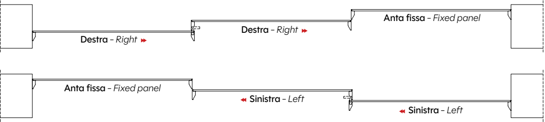
Tre ante in luce con trascinamento - Three sliding panels within the opening with synchronized movement
